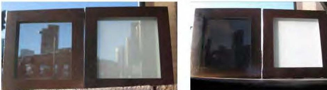
Figure 5. Assorted Views of RavenWindow and RavenLight Filters in the Cold (Transparent) and Hot (Reflective) State.
