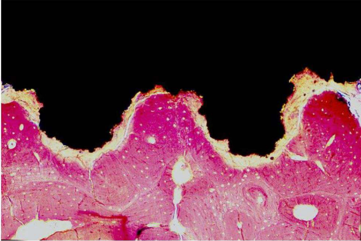
Figure 27. Photomicrograph of Titanium Metal (Appears Black in This Photo) in an Intimate Integration With Living Bone. The intersection of the two materials shows a thin barrier layer and then healthy tissue very close to the metal. It does not show inflammation or scar tissue formation.
