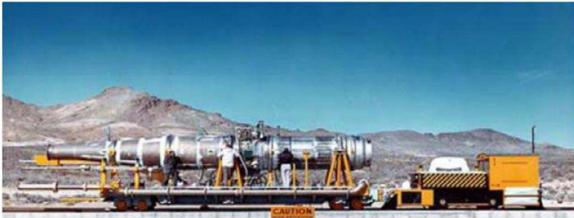
Figure 2. Tory-IIC Ready for Testing (courtesy LLNL)
