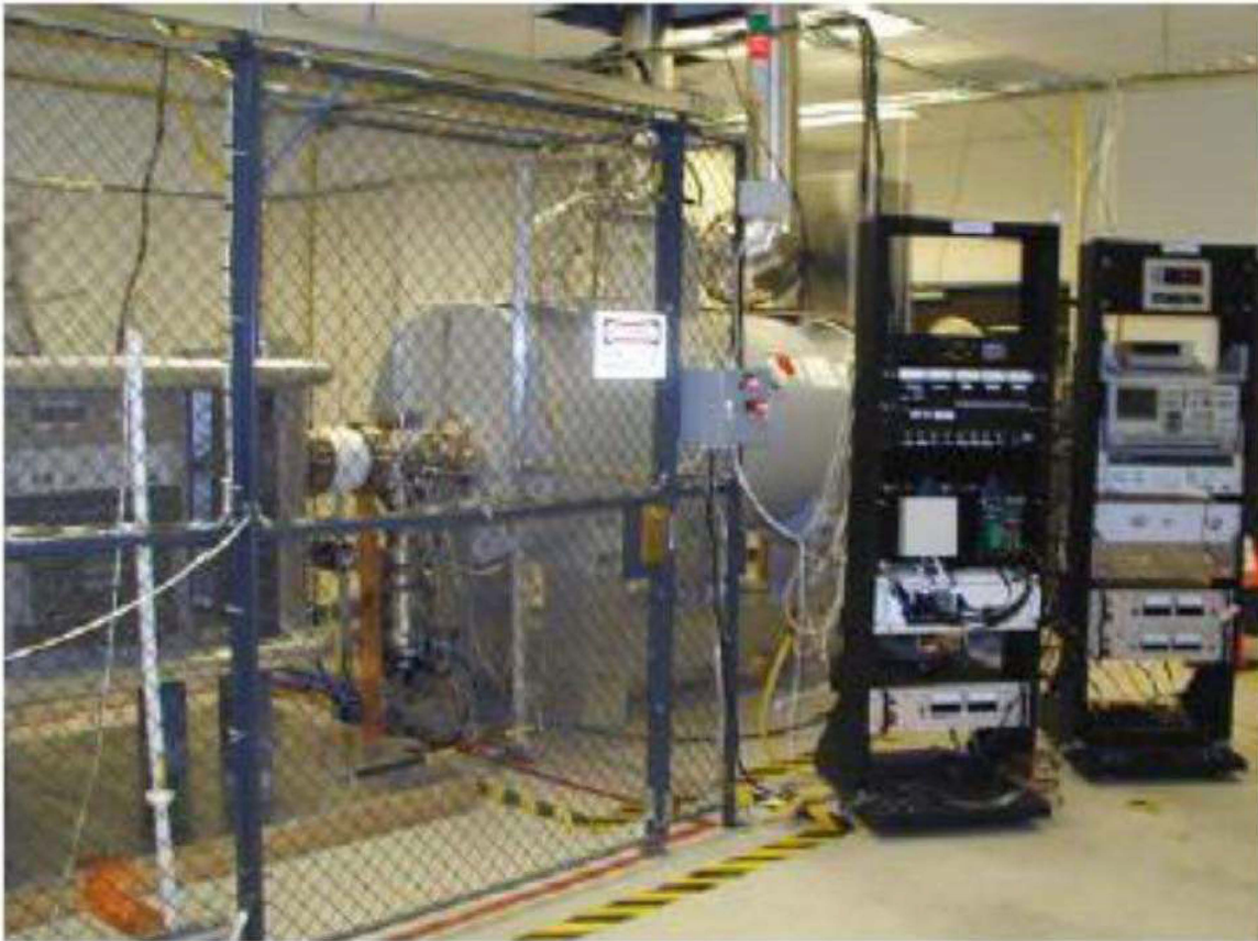
Figure 19. Penning Trap With Trapping Volume of 1,000 Cubic Centimeters (center), Injection Apparatus (left) and Controls (right) (courtesy Positronics Research LLC) 68
