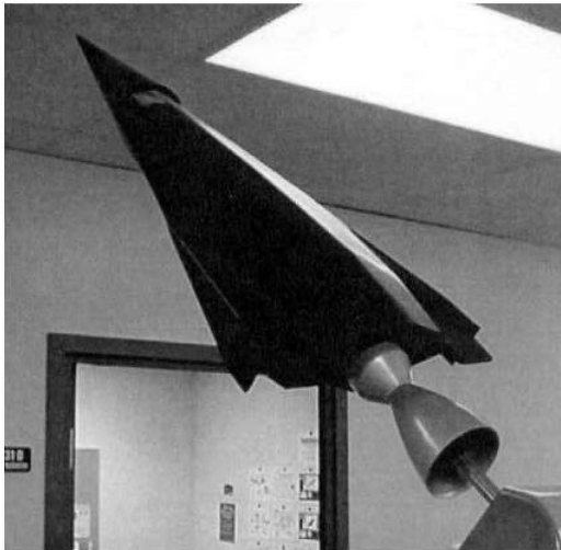
Figure 27. Boost-Glide Strategic Vehicle With Pratt & Whitney XLR-129 Rocket Engine Installed, Circa 1964
