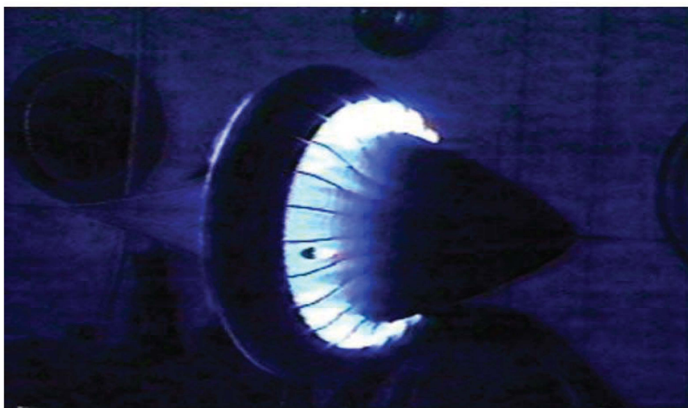
Figure 5. Lightcraft Undergoing Horizontal Guide-Wire Flight Test (courtesy of F. Mead, AFRL/PRSP, Edwards AFB, CA).
