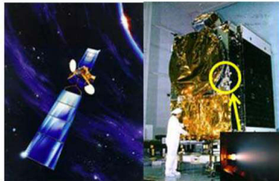
Figure 11. Electrothermal Arcjet Thruster on Satellite. Lockheed Martin Series 7000 Comsat with Aerojet 1.8-kW Arcjet thrusters (insert photo) for north-south station keeping.
