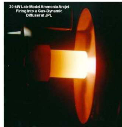
Figure 1. Electrothermal Arcjet Thruster. Photograph of a 30-kW arcjet thruster being tested at the Jet Propulsion Laboratory. 13
